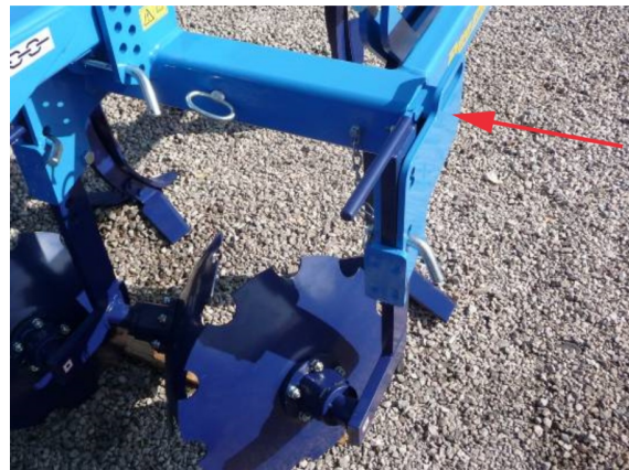
Fig. 6 - Rear twin roller in the transport position
