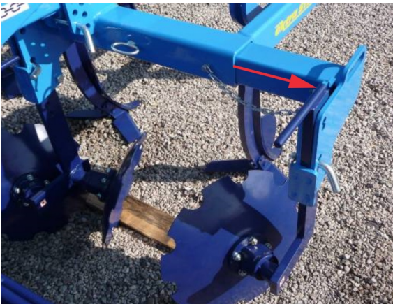
Fig. 5 - Rear twin roller in the working position
