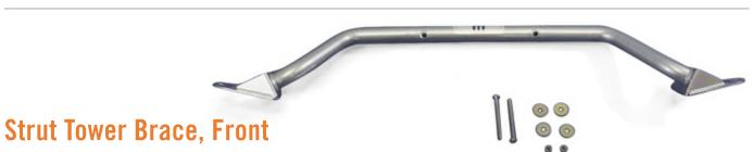
This transverse-mounted horizontal strut tower brace will enhance structural rigidity, steering response, directional stability and vehicle handling. Made of heavy-duty steel and supplied with all applicable mounting hardware. Not compatible with vehicles equipped with "Shaker" Hood Scoop or SRT® Hellcat engines.
