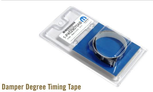
Improve timing accuracy with this damper degree timing tape. Marked in 90° increments. Self-adhesive strip adheres to the crank vibration damper for clear identification of marks. Permits initial total spark advance up to 60° instead of only 10°-15° as on chain case timing tab.
