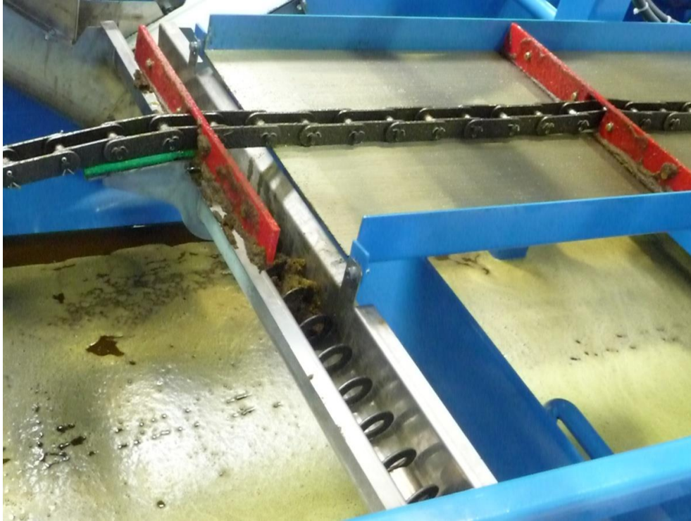
Figure 3 - Transfer of sediment into the spiral conveyor
